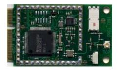
S3MPE radio module enables the implementation of complex wireless sensor networks but can also be used for simple telemetry applications
